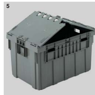
5 180 litres – Ref. 1B650 Ext. dim.: L 865 x w 610 x h 500mm Ext. dim.: L 34.1 x w 24.0 x h 19.7" Int. dim.: L 760 x w 495 x h 460mm Int. dim.: L 29.9 x w 19.5 x h 18.1" Nested height: 183mm/7.2" Weight: 8.6 Kg/18.9 lbs. Colour: light grey
