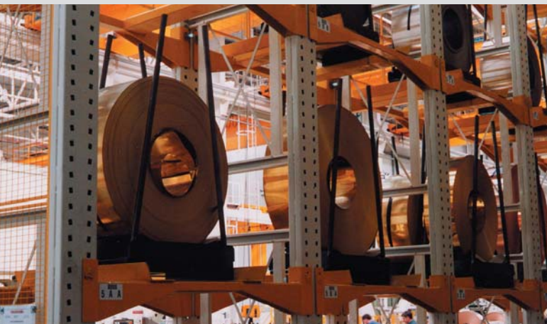
Copper alloy storage: 12 tonnes per level on adjustable cantilever racking
