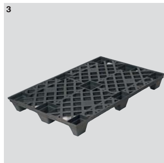
3 Ref. 3D003 pallet with 9 feet ventilated deck with 5mm collar Dim.: L 1,200 x w 800 x h 144mm Dim.: L 47.2 x w 31.5 x h 5.7" Nested height: 45mm / 1.8" Wt: 7.8 Kg/17.2 lbs. Colour: dark grey Supplied in quantities of 50 pallets
