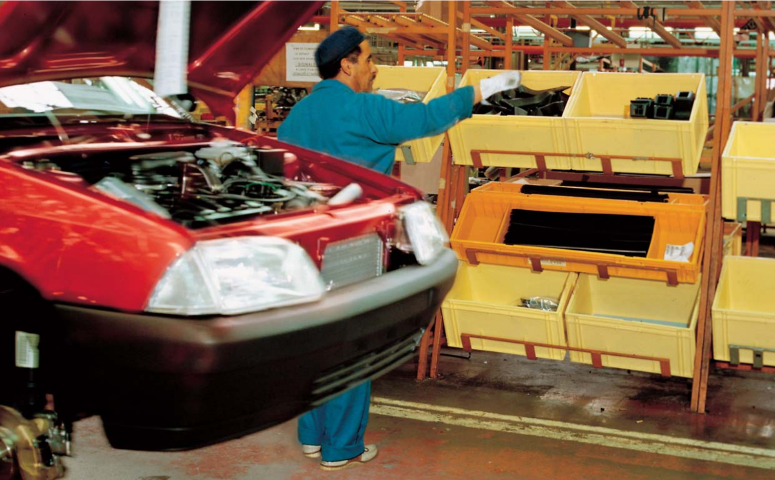
Automotive industry: containers developed for just-in-time distribution of components (Odette 20 kg containers and Galia containers).
