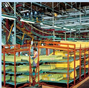
Automotive industry: reusable packaging suitable for rapid just-in-time rotation (Odette 20kg containers).
