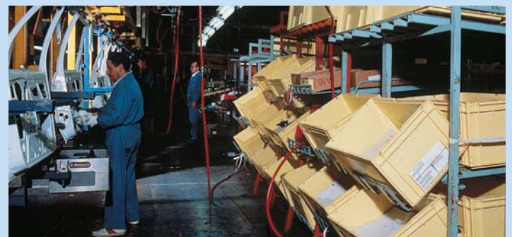
Easy access to component parts while keeping the production line clear of obstruction (Odette 20kg containers).
